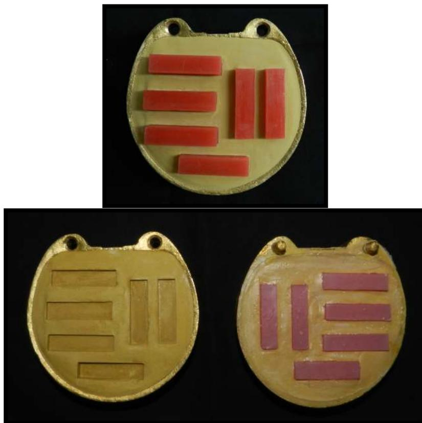
*Figure 3: Surface pre-treatments with 35% hydrochloric acid etching*
