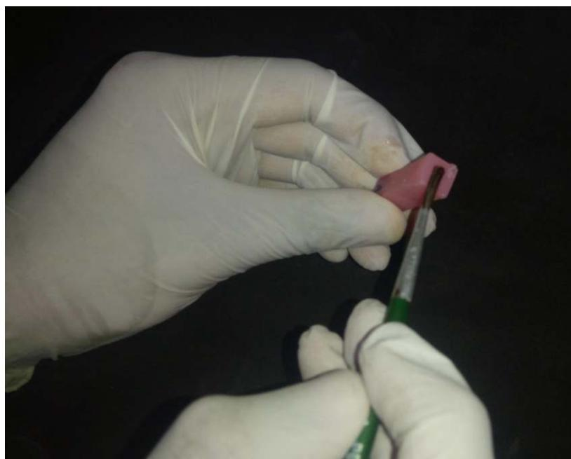
*Figure 4: Surface pre-treatments with 110  $\mu\text{m}$   $\text{Al}_2\text{O}_3$  air abrasion*
