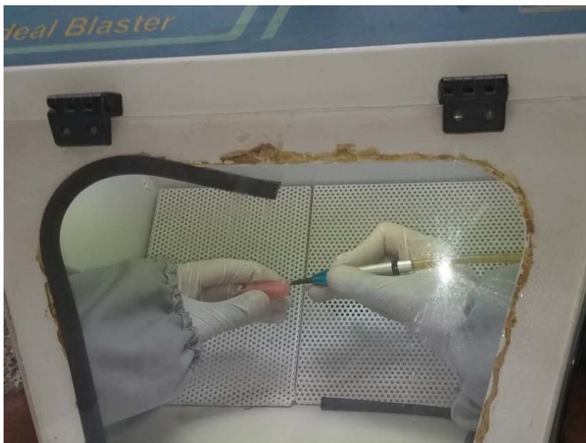
*Figure 5: Fabrication of test specimens for Molloplast-B subgroups*
